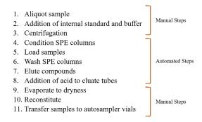
Figure 4 Description of manual and automated sample preparation steps
