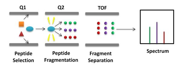
Figure 11 - Schematic of a Quadrupole Time-of-Flight mass spectrometer. Bottom — MS/MS spectra generation through peptide isolation in quadrupole one (Q1), fragmentation in the collision cell (Q2), followed by separation by the TOF mass analyzer.
