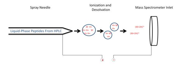
Figure 8 - Electrospray ionization source. Peptides eluting into the source are charged, dried, and travel into the mass spectrometer inlet.
