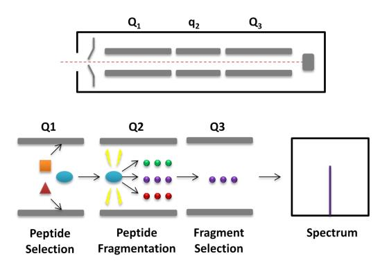
Figure 12 - Schematic of a triple quadrupole mass spectrometer. Bottom – MS/MS spectra generation through MRM mode with peptide isolation in quadrupole 1 (Q1), fragmentation in the collision cell (Q2), product ion isolation in quadrupole 2 (Q33.
