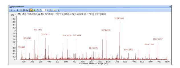
Figure 36 - In a Q-TOF assay, inclusion list precursor ions are only isolated in the first quadrupole (Q1). After the isolated precursor ions are fragmented in the collision cell all product ions reach the detector. These fragments generate a complex fragmentation spectrum which can be analyzed to confirm the presence of a particular protein biomarker in a database.
