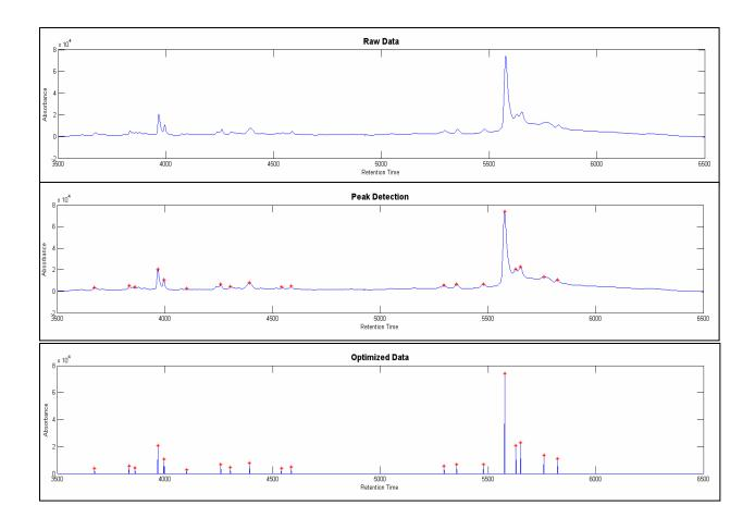
Figure 17 - Application of a protein peak identification algorithm to raw hydrophobicity data (top) generated from a single first-dimension ProteomeLab™ PF2D fraction. Protein peaks are called based on the point at which the slope changes from positive to negative or the point where a derivative changes signs (middle). Once identified, called protein peaks are used to create a normalized representative dataset from which > 99.9% of the underlying noise has been eliminated (bottom).
