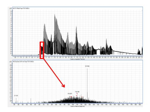
Figure 26 - Column overloading with saliva on a fast 22 minute gradient generating irresolvable MS scan.
