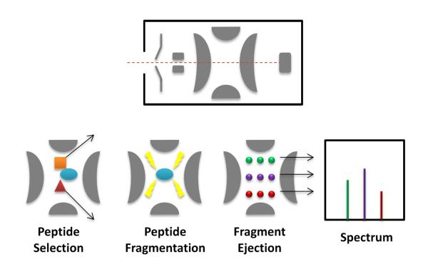
Figure 10 Top – Schematic of an ion trap mass spectrometer. Bottom – MS/MS spectra generation through peptide isolation, fragmentation, and ejection from the ion trap.
